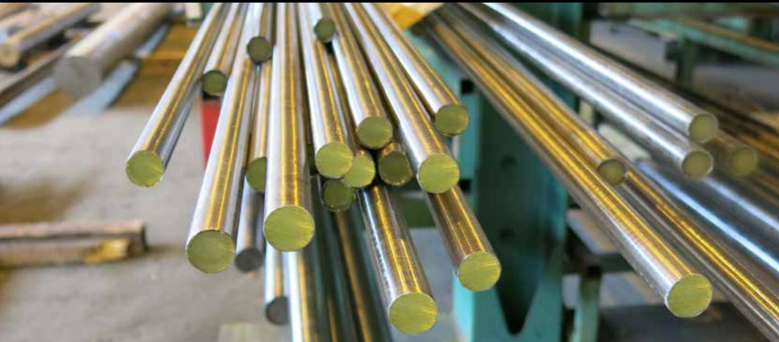
**Toolox in round bars, delivered heat treated to high tensile strength levels of typically 1450 MPa, represents entirely new possibilities for product design. The need for heat treatments on standard steel grades is eliminated and the time-to-market becomes shorter.**
