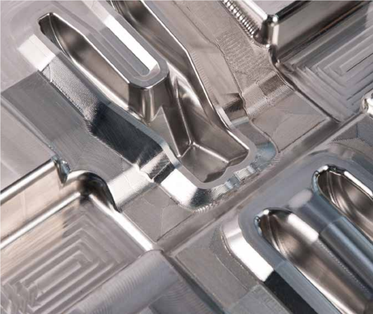
▲ GSF hammer die with fine engraving, performance increased by currently 47% compared to 1.2714
