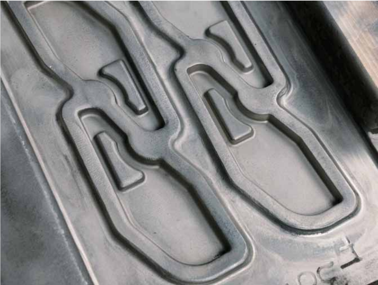
▲ GSF hammer die with fine engraving, performance increased by currently 47% compared to 1.2714
