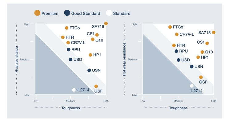
Good standard: Standardised alloy concept (ISO), but very well executed by KIND & Co. Well balanced material quality, therefore often a good selection for many intended uses. Premium hot work tool steel with property combinations tailored to meet the intented use with maxium efficiency.
