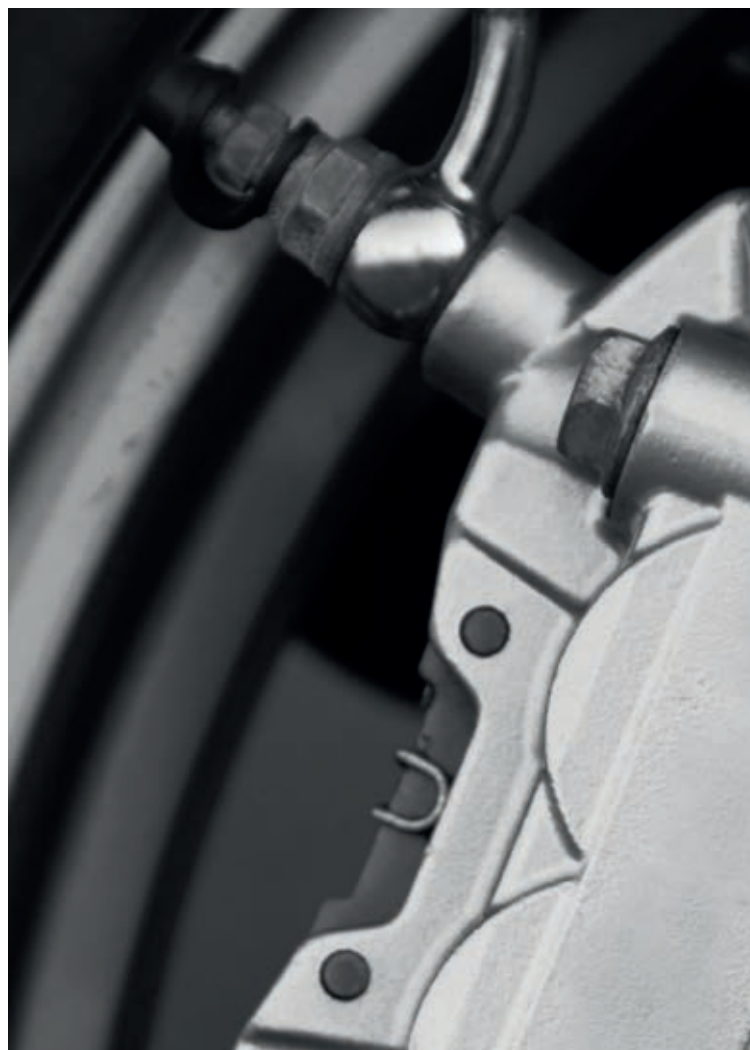
▲ Brake caliper of a motorcycle in aluminum alloy
