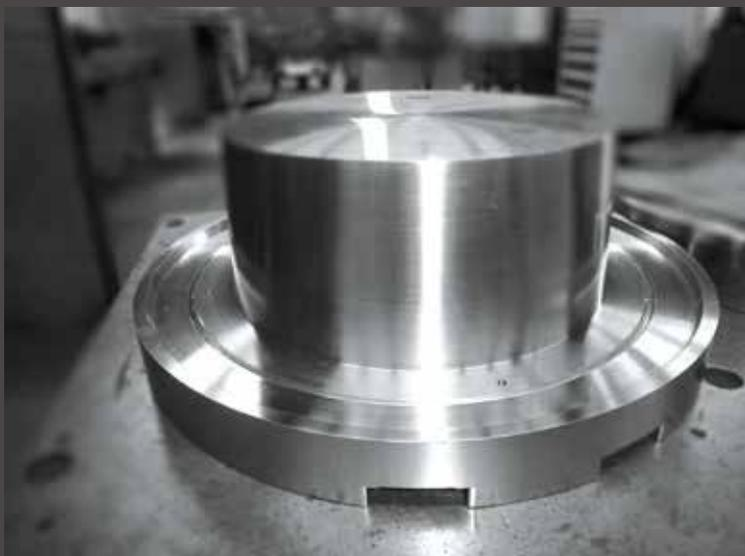
Rubber mould component after machining ▲
