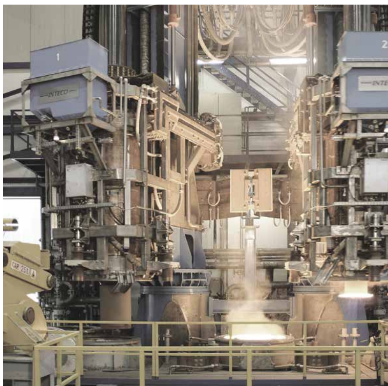
◀ Electro-slag remelting process (ESR)
